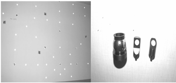
(a) 统计像面上误差的靶点场 (b) 跟踪仪和视觉系统的转换附件 (a) Target field used to statistic (b) Transmission accessory between laser tracker and computer vision system
